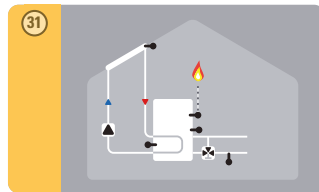
Solar with thermostat and return flow increase
